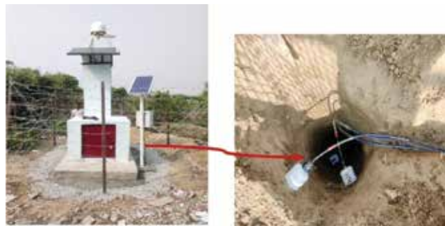
Figure 3. GPS-Soil Moisture Observatory at JNV, Aurangabad, Bihar (Left). Three Digital Hydra Probe soil sensors installed at three distinct soil horizons (Right).
