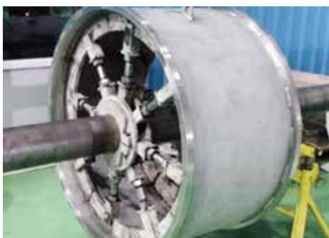
Fig. 2: Vacuum vessels under fabrication (INOX India, Vadodara)
