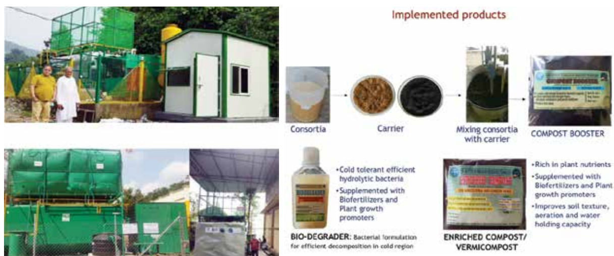
Fig: Bio digester (capacity 250 Kg/day) functional at Baijnath, HP and Gyalshing, West Sikkim
