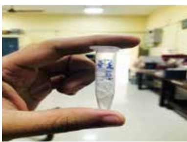
Electrospun pullulan- prebiotic-lyoprotectant fibres loaded with L. rhamnosus
