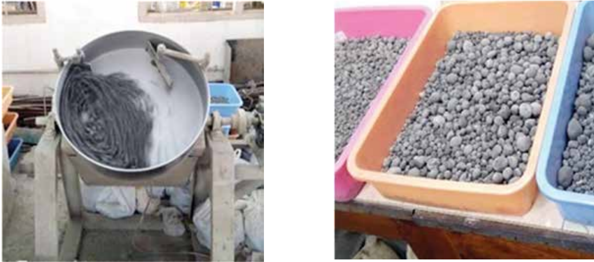
Fig: Laboratory trial production of Geopolymerized Aggregates
