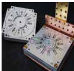
Ring resonator coupler for superconducting qubits
