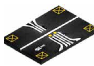
Gate-defined double quantum dot system
