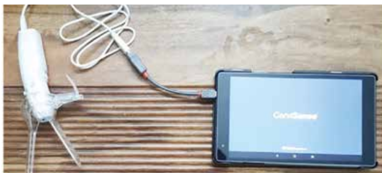
Fig 4. Cervisense: portable, non-invasive point-of-care imaging device
