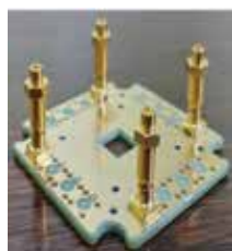
2D microwave packaging for superconducting qubits
