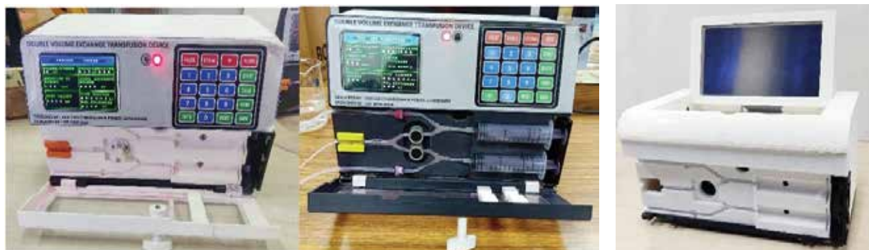
Fig: Double Volume Exchange Transfusion front view showing screen and keypad
